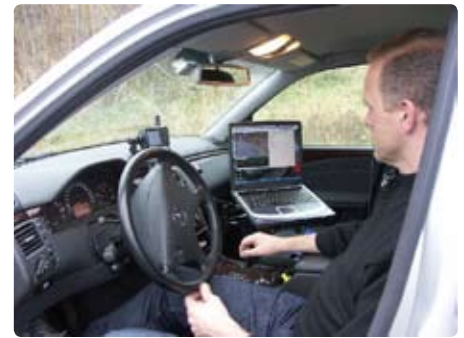
The PC is connected to the GPS and the trip counter
